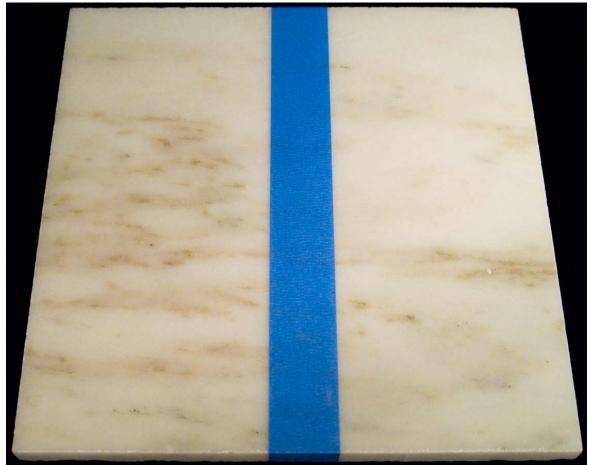
The face of this stone has been treated with Comet and sealed with 511 Impregnator. The left side will be stained and refinished; the right side will be left alone.
